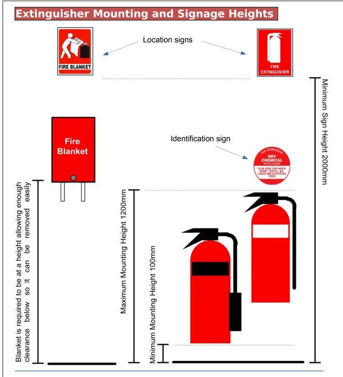
Location signs must be fitted at a minimum height of 2 metres above floor level, or in a location and height that makes it most apparent to a person of average height approaching the extinguisher(s) or fire blanket.
